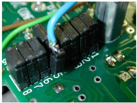
The connection to the mic configuration header – only a single wire is used, the ground connects through the K2 ground system. Note that I used pin 5, use whichever pin is available for your setup.
