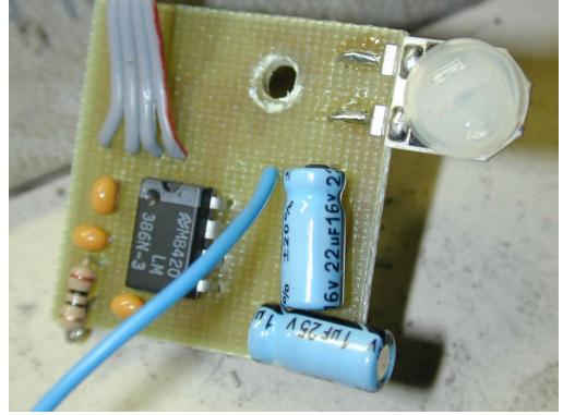
The fixed audio board with components laid flat so it can be mounted between the FP and CB in the K2.
