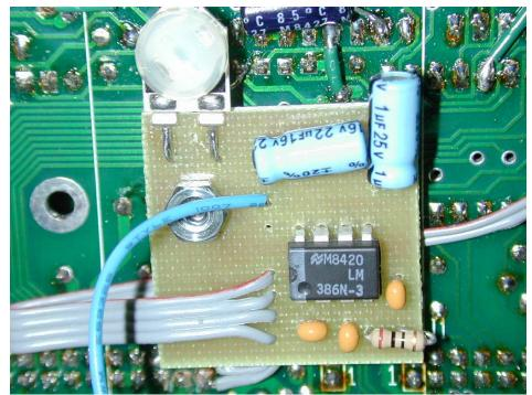
Fixed audio board mounted on the back of the Control Board – there is an unused mounting hole in the CB that I used – short spacer between the boards (drill your own mounting hole in the fixed audio board.
